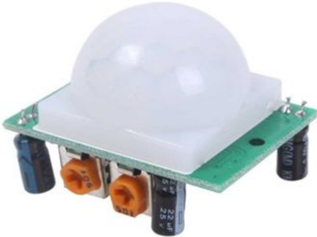
Figure 6 – “PIR Motion Detector Sensor Module HC-SR501” by electronicscomp
